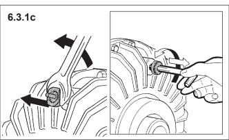
To fill and calibrate the horizontally mounted fluid coupling, observe the following steps:
