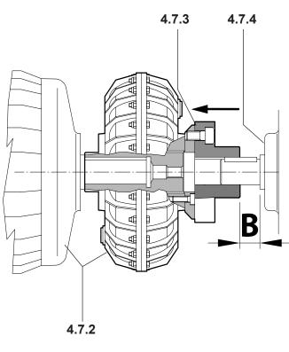
The ROTOFLEXI flexible coupling is an accessory to the ROTOFLUID ALFA couplings and it is anchored on the farthest fluid coupling side for keying it on the reduction gear (standard assembly) or on the motor (reversed assembly). To install it correctly, please observe the following steps:
