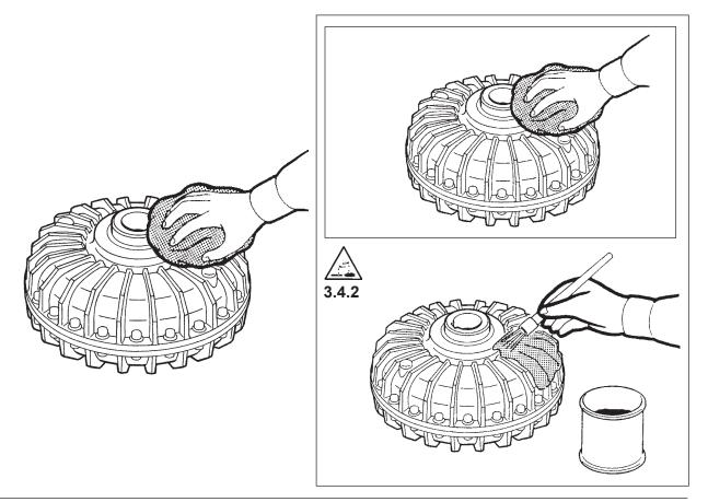
The pre-assembly steps vary according to the location, where the coupling shall operate; to prepare it for assembly, observe what follows:
