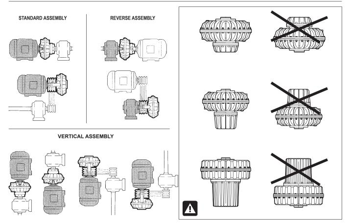
The standard ROTOFLUID coupling (standard production) is delivered with hollow shaft and keyseat according to DIN 6885 standard for UNEL MEC motors. The keying of the coupling (hollow shaft side) can be carried out on the motor (electric or endothermic) as well as on the machine driven end, according to the specific instructions reported on both the Identification Plate and the TECHNICAL DATA SHEET OF THE FLUID COUPLING.
