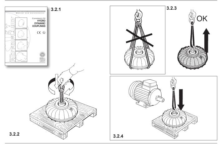
To handle the fluid coupling without its package, it is necessary to follow this procedure:
