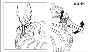
The first filling must be carried out on the bench with the coupling installed on the motor and its axis positioned horizontally (see section 6.3).
