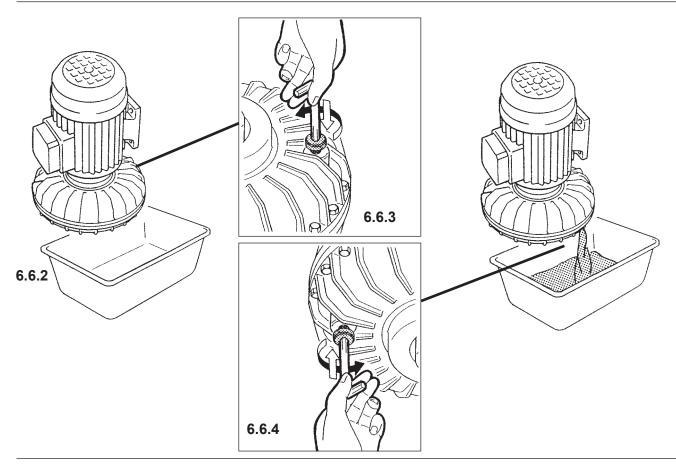
The first transmission oil change must be carried out after 2000 operating hours and later every 4000 operating hours. The use of the coupling in particularly dusty environments also shortens the planned intervals and requires oil replacement every 1000 operating hours. The oil must be changed even after a partial start-up of the motor, so that impurities are suspended in the oil. After that, please follow the described procedure:
