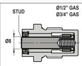
TE = Expandable Trip Plug (trigger temperatures 96°C [204.80°F], 120°C [248°F], 145°C [293°F] e 180°C[356°F]).
